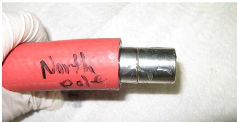
Image 2: Photo of static, neodymium cylinder magnets inserted into the sprayer water hose.
