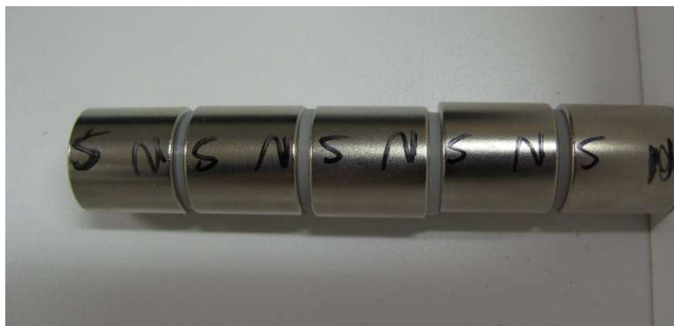
Image 1: Photo of static, neodymium cylinder magnets with plastic washers inserted between each magnet.
