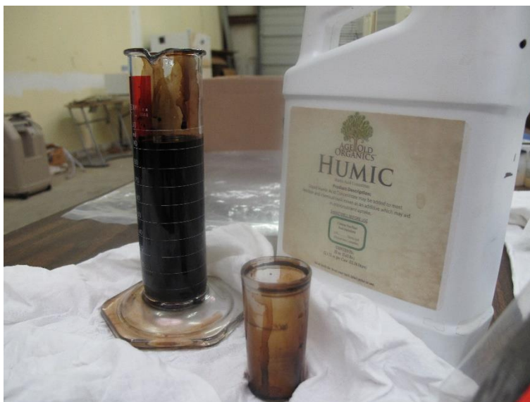
Figure 3: Image of humic acid used as an organic challenge by adding it to the five-gallon water tank at 0.025 or 0.05% v/v.
