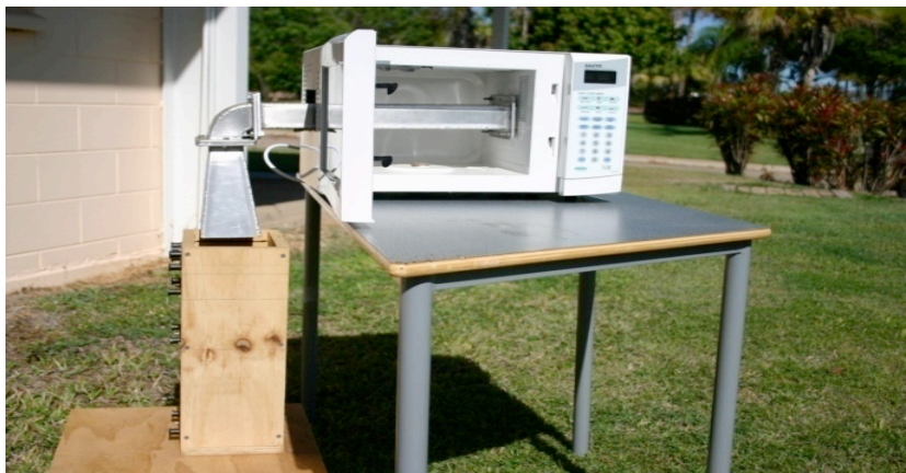
Figure 2: Microwave prototype system based on a modified microwave oven, including wooden box used for soil bacteria study [Source: 9].
