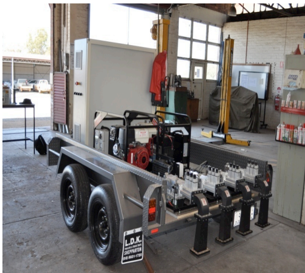
Figure 1: Trailer mounted four by 2kW microwave system to treat weeds and soil.
