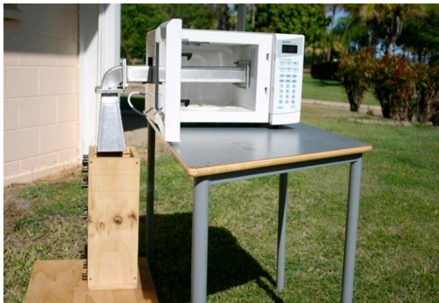
Figure 2: Modified microwave oven with a waveguide and horn antenna arrangement to treat weeds and soil [Source: 20].
