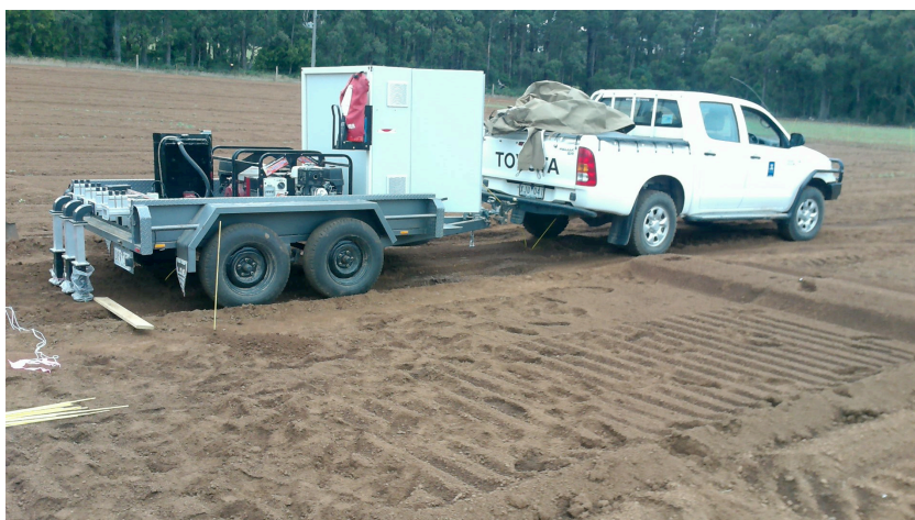
Figure 10: Four by 2 kW microwave trailer prototype in the field.
