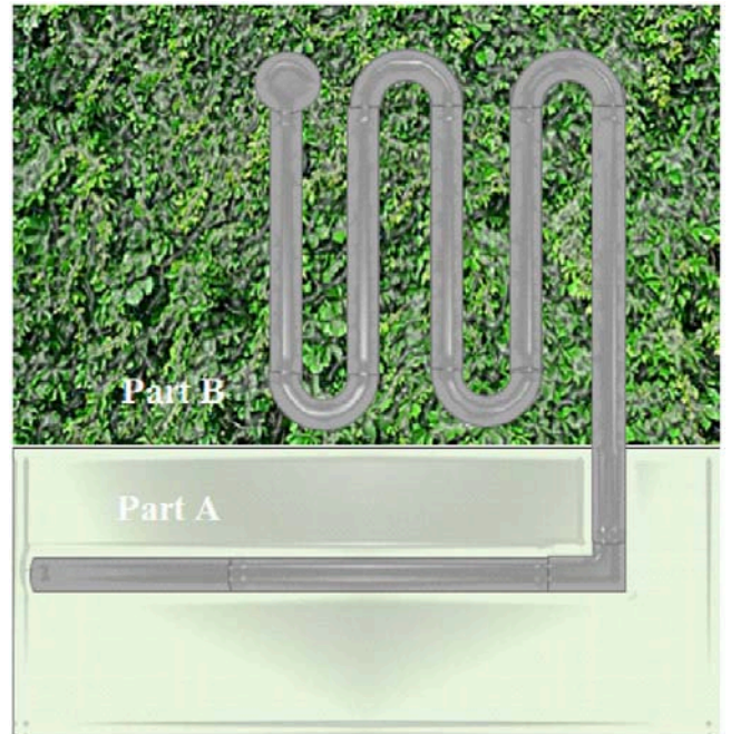
Figure 4: Schematic of the modelled system consisting of an earth-air heat exchanger (EAHE) assisted by a green wall (GAHE).
