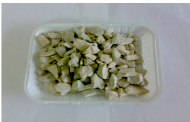
Picture 2: Ash (spent shale after calcination at 950 °C).
