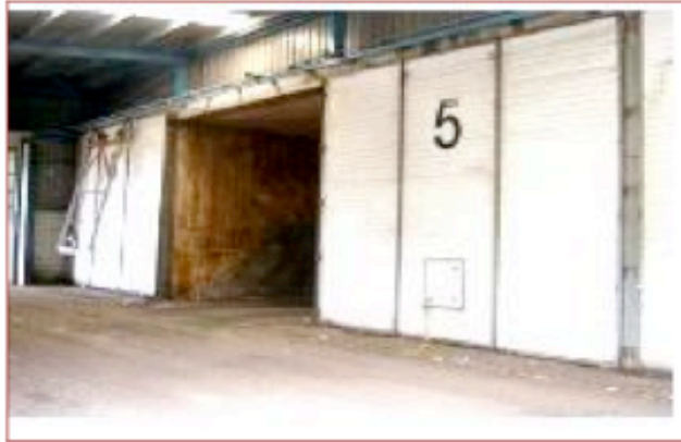
Figure 5: Batch-wise dry anaerobic bioreactors for treating MSW organic fraction.
