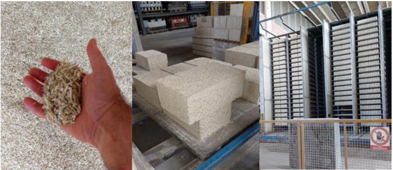
Figure 9: Showing hemp shives added to lime / water binder to manufacture hempcrete masonry blocks. Senini-Tecno Canapa northern Italy [Source Author].
