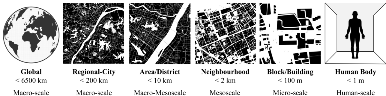
Figure 7: Classification of investigation scales in studies of urban climatology and urban physics (drawn by authors based on [44]).
