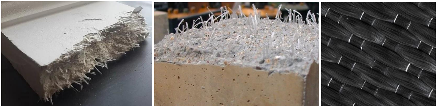
Figure 3: High-performance fiber-reinforced concrete (HPFRC) and carbon fiber-reinforced polymers (CFRP) enhance strength, durability, and flexibility in complex architectural structures. Sources: [37].
