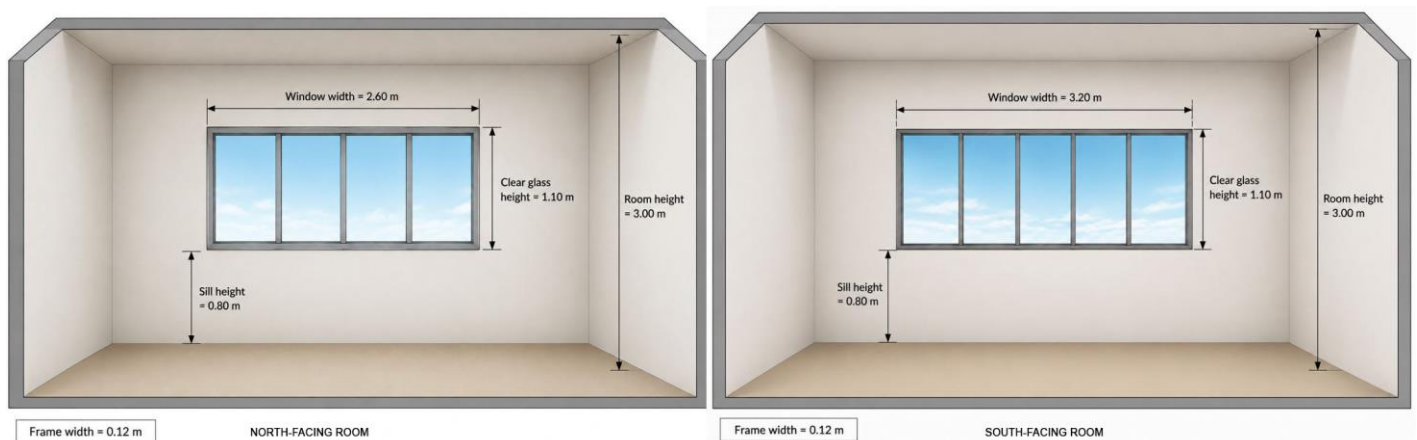
Figure 2: Window configuration and dimensions of the selected patient rooms.
