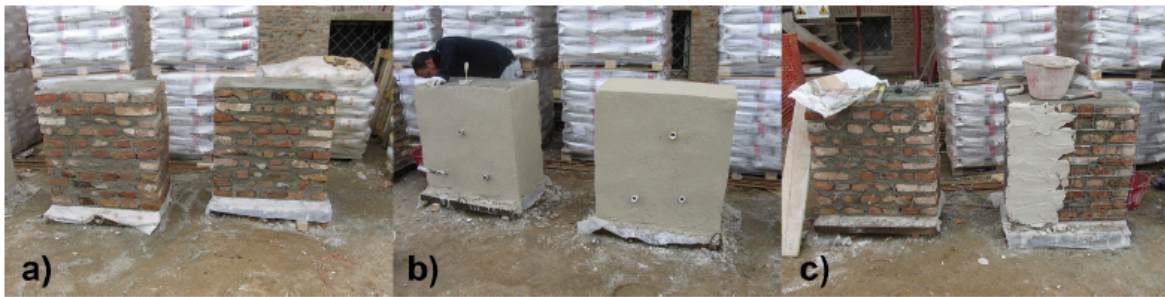
Figure 6: (a) Original masonry specimens; (b) masonry specimens strengthened by injection technique; (c) masonry specimens strengthened by jacketing wall technique.
