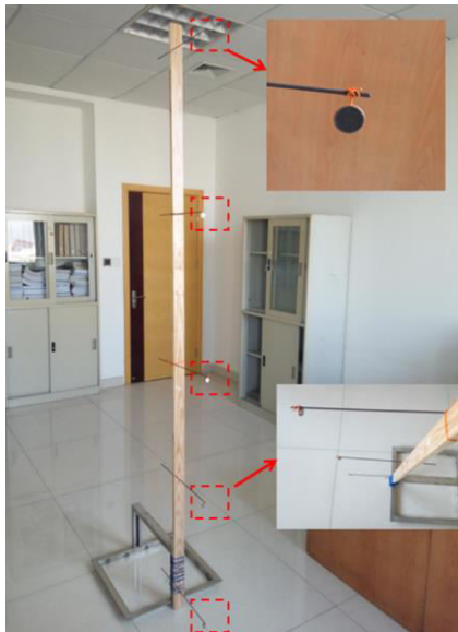
Figure 11: The locations of the iButton temperature sensors in test room study.
