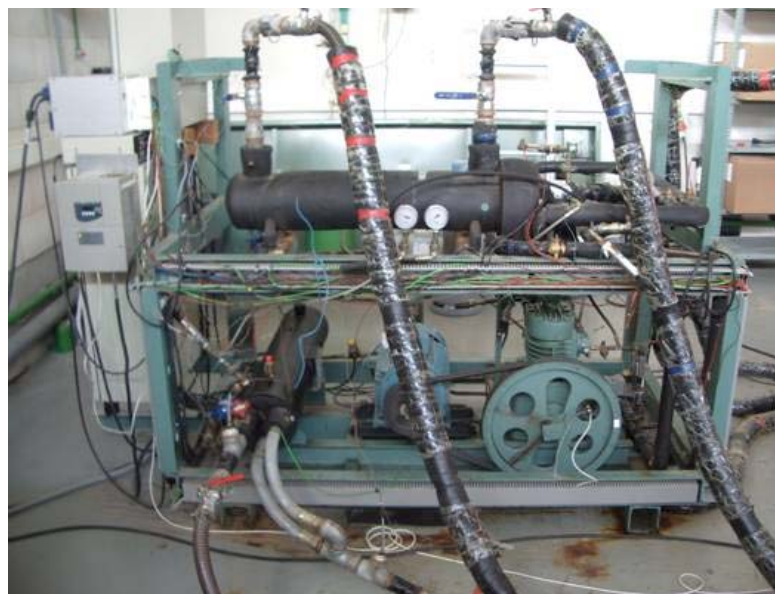
Figure 1: Test facility of the vapor compression system.
