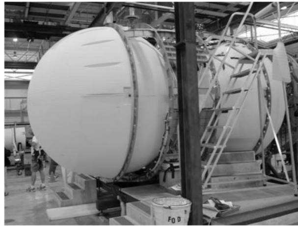
Figure 6: Actual image of a liquid hydrogen spherical tank utilizing SOFI adiabatic technology.
