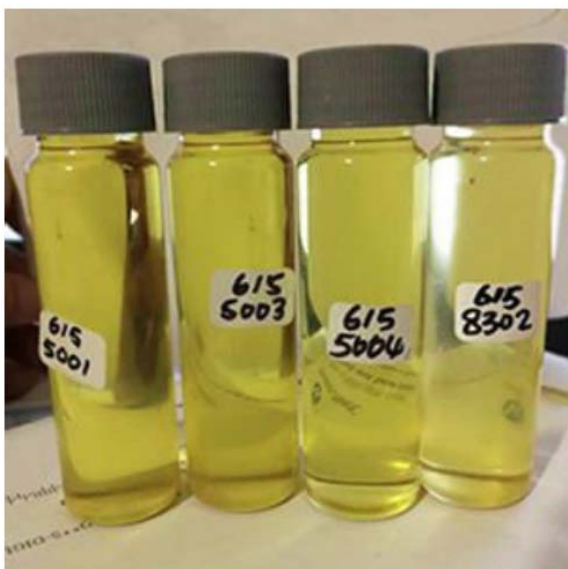
Figure 17: Liquid product from pyrolysis of NMF from scrap PCB.
